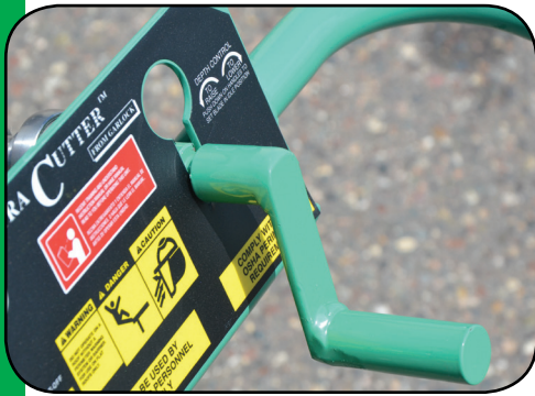
Depth adjuster in travel mode Press down on handlebar for travel mode
