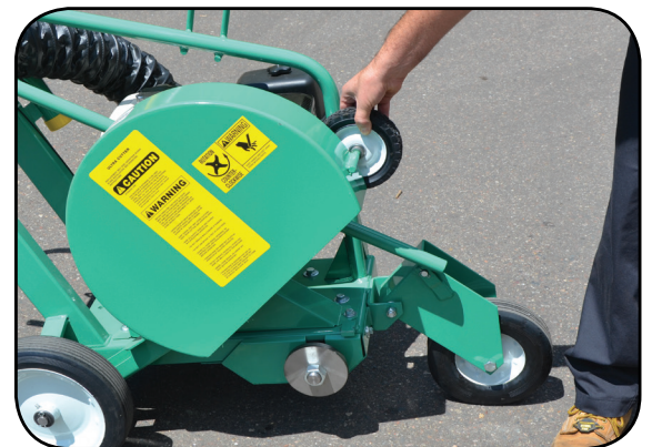
Easy No-Tool access to blade with lift up shroud
