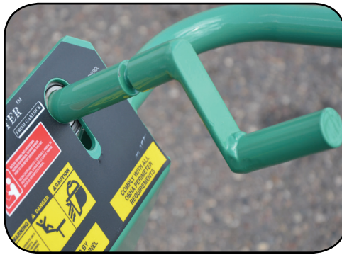
Depth adjuster in work mode Lift up on adjuster to work.
