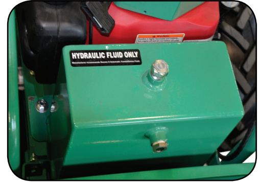
Large hydraulic tank with sight gauge.
