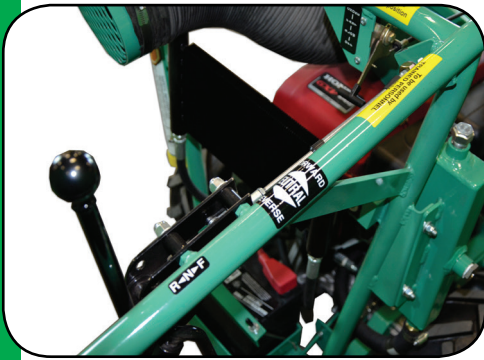
Smooth Hydrostatic drive with forward/reverse lever at handle for safety.
