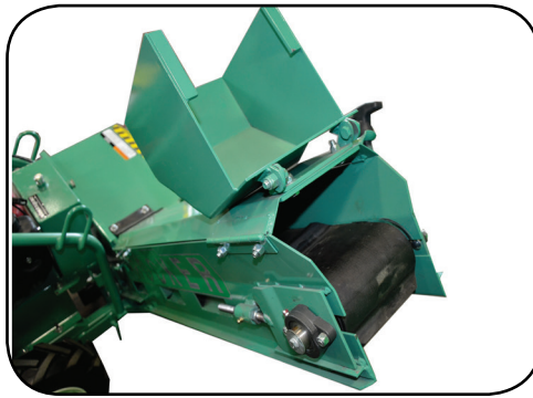
Rugged belt delivery system with access door.
