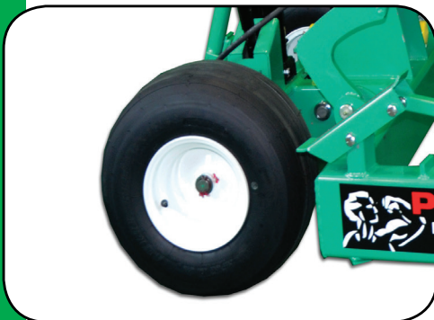
Large smooth air filled tires provide stability and spread surface load.
