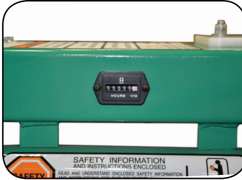
Hour meter for maintaining service intervals.
