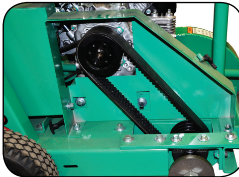
Rugged belt drive system with quick access panel.
