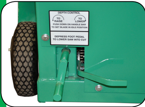
Depress foot pedal to lower saw into cut. Press down on handlebar to raise saw.
